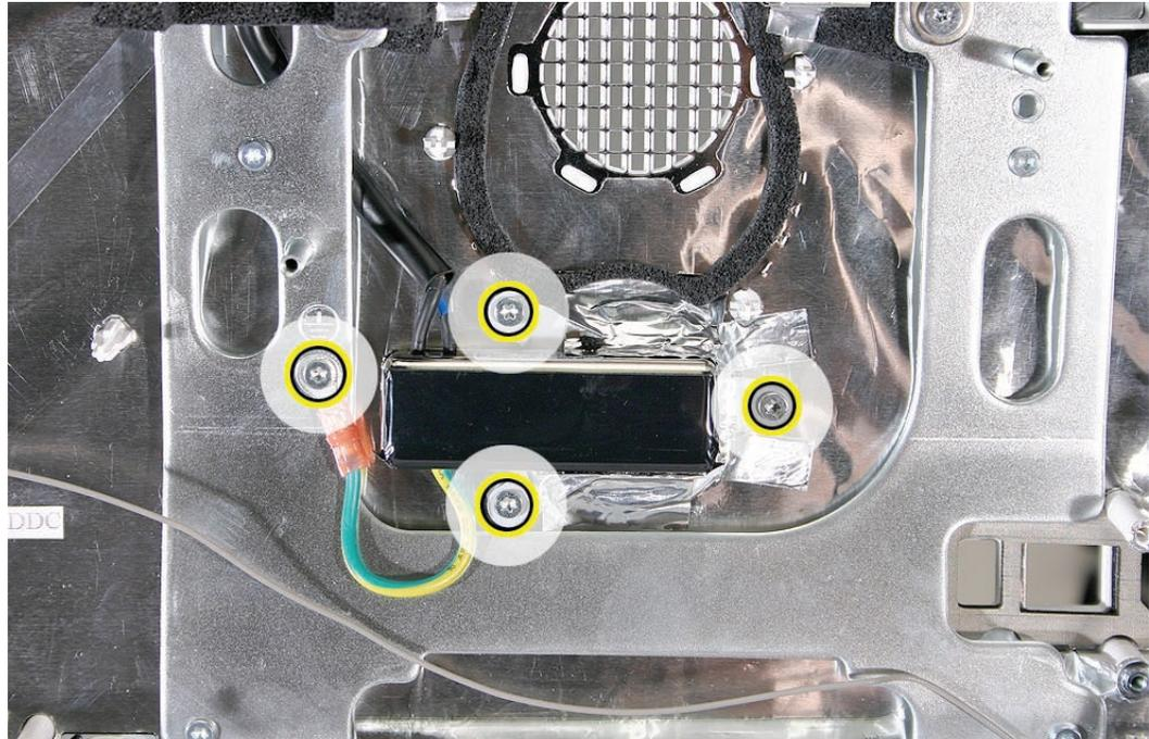
3. Peel the EMI tape off the power inlet.
