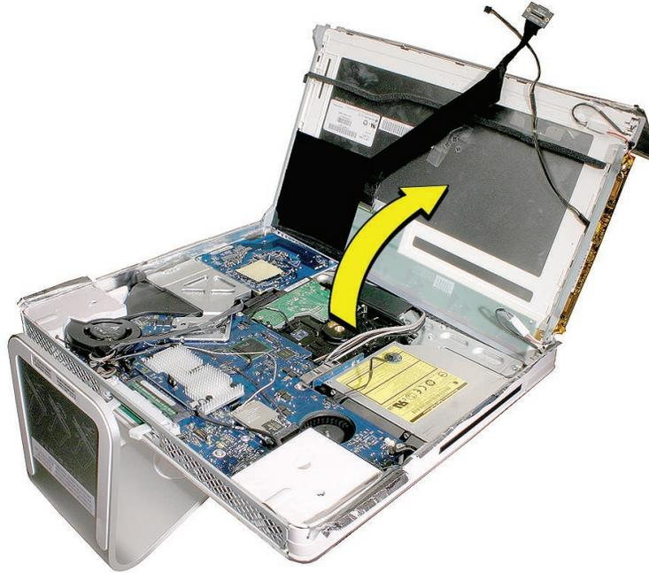
**Note:** If replacing a bad LCD display, you will need to remove the lower EMI shield (if still attached), the display panel mounting brackets, and the LVDS cable as follows.
